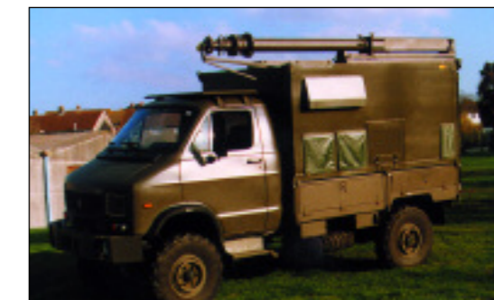
SCAM 21 - Roof mounting system
